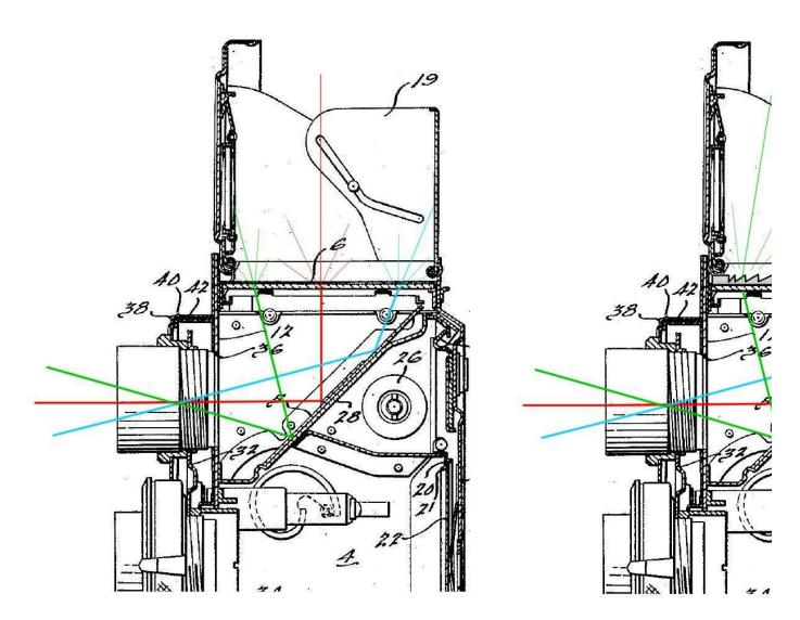
On the left is a TLR with a plain groundglass, on the right the same TLR with a Fresnel lens added. The length and weight of the colored lines reflects the amount of light that each line
